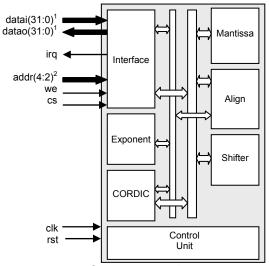
**Exponent** – performs operations on exponent part of number. The addition, subtraction, shifting, comparison and conversion operations are executed in this module. It contains exponents and work registers.
